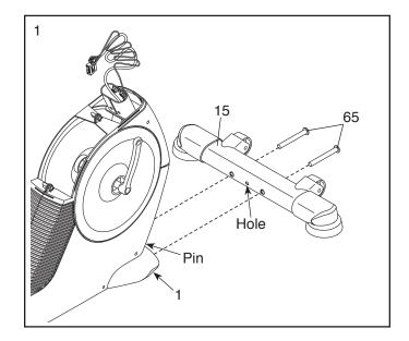
While a second person lifts the rear of the Frame (1), attach the Rear Stabilizer (16) to the Frame with two M10 x 105mm Screws (65).
